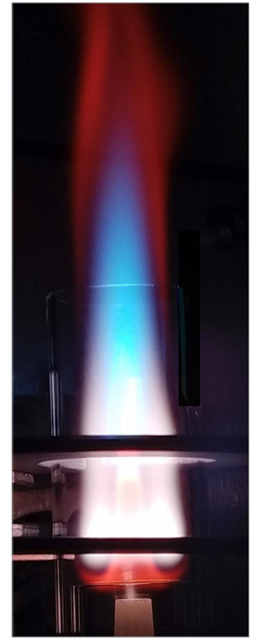
Figure 6. Yttrium plasma with the blue color showing the normal emission and the red color showing the cooler tail plume.
