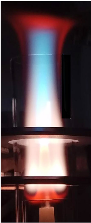
Figure 4. Yttrium plasma with the blue color showing the normal emission and the red color showing the cooler tail plume displaced by the air shear gas.
