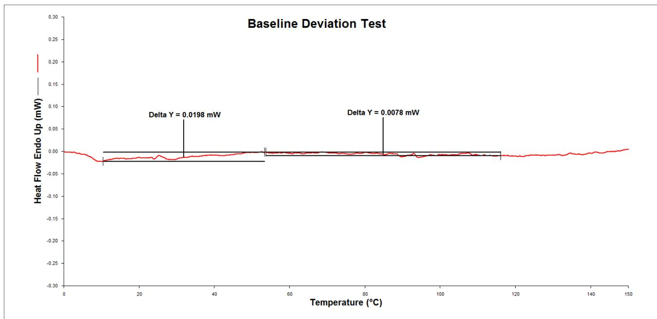
Figure 2. Baseline Deviation Graph calculation from 0 to 150°C.
