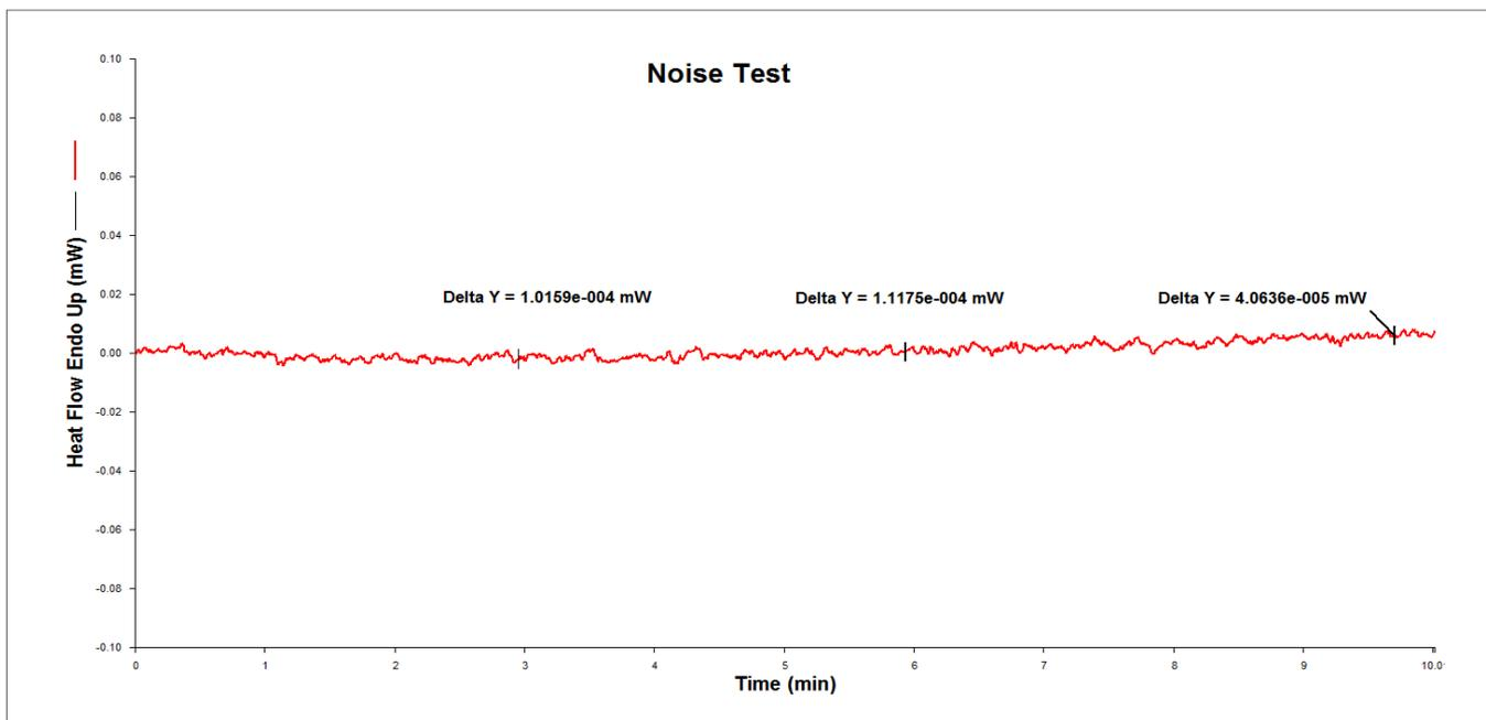
Figure 4. Noise test thermogram.
