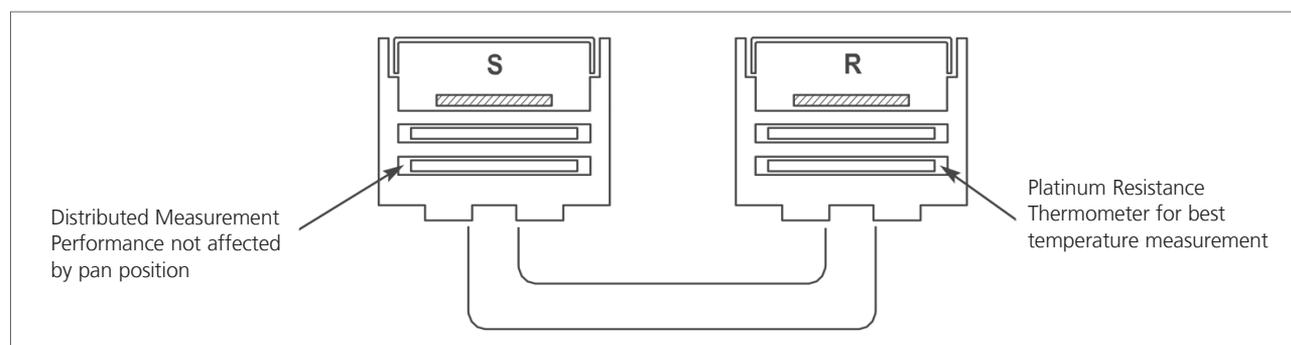
Figure 1. Double Furnace DSC design
