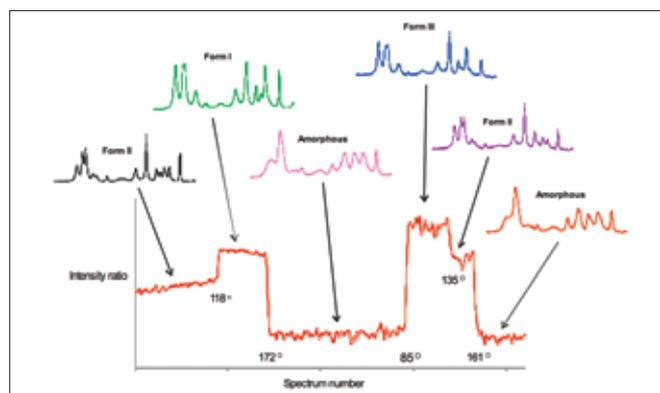
Figure 4. Thermogram and spectra from heating acetaminophen Form II.
