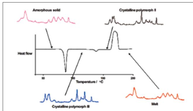
Figure 3. Raman spectra (1700-1100 cm<sup>-1</sup>) from a DSC run.
