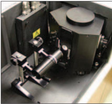
Figure 4. Beam condenser fitted in the cradle holder.
