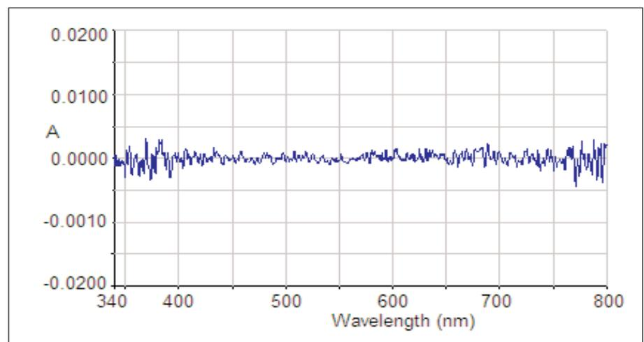
Figure 7. Baseline using a 1mm aperture and 1% T Reference Beam Attenuator.
