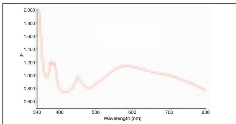
Figure 10. Absorbance spectrum of synthetic blue sapphire.
