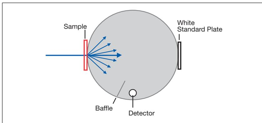
Figure 1. Integrating sphere for transmission measurements.
