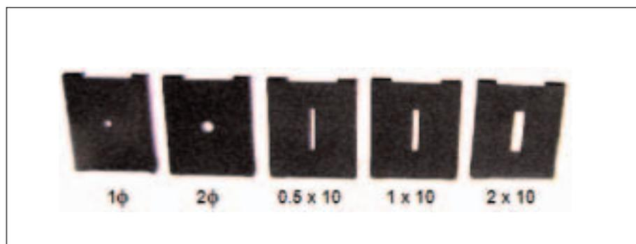
Figure 2. Beam apertures (sizes in mm).
