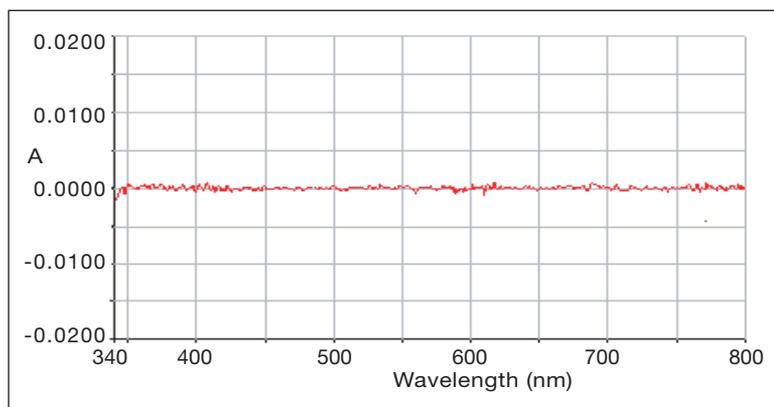
Figure 8. Baseline using a beam condenser.
