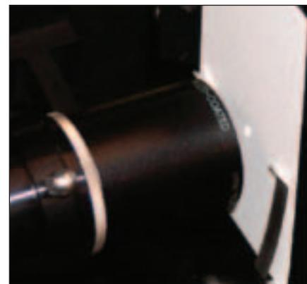
Figure 3. 1 mm beam spot using the condenser.
