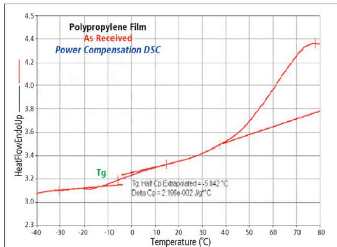
Figure 2. Enlarged view of T<sub>g</sub> of as received polypropylene film sample.
