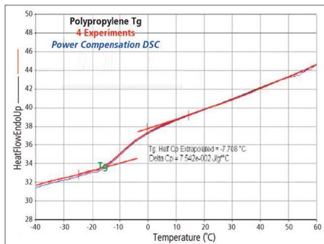
Figure 4. Reproducibility of T<sub>g</sub> of reheat polypropylene sample showing overlay of four (4) DSC experiments.
